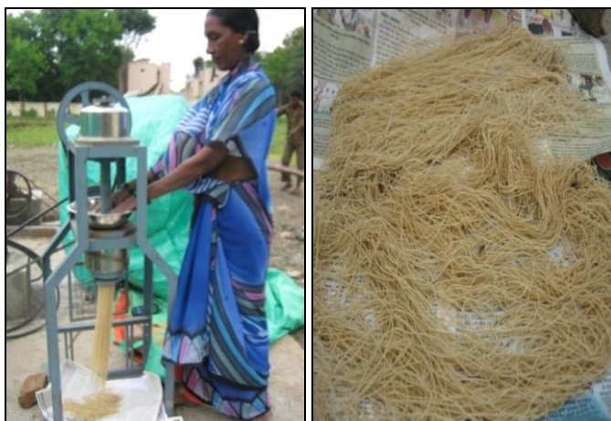
Shevai Obtained from Bullock Operated Power Transmission System
