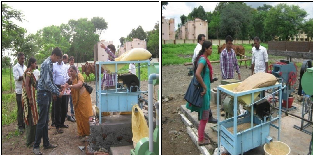
Plate 2, 3: Grain cleaner cum grader in rotary mode operation
