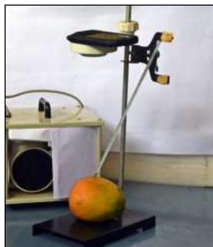
Fig 2: Experimental setup for determination of thermal emissivity using thermal imaging technique.
