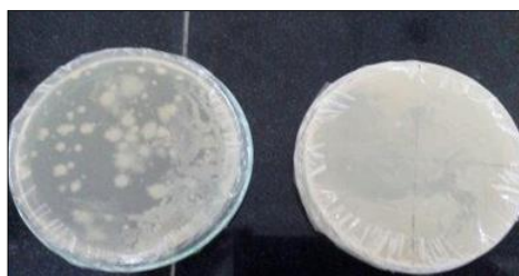
Fig 3: Effect of chlorination on microbial water Untreated & treated sample grown NA media plates.
