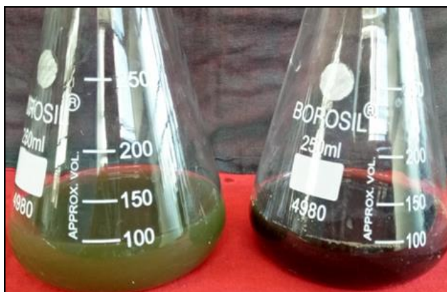
Plate 1: Plant extracts, (A) before addition of AgNO 3 , (B): after formation of silver nanoparticles
